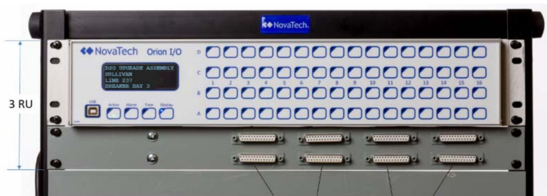
DB25 connectors wired to Orion I/O input cards
