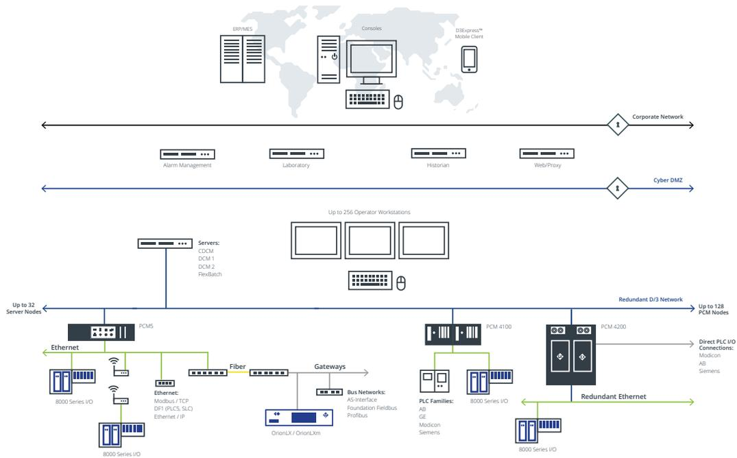
The D/3<sup>®</sup> Distributed Control System (DCS) is a completely scalable solution to meet your current and future process control needs. NovaTech D/3 products are currently employed by customers with as few as 50 and as many as 40,000 tags — with room to grow to over 100,000 tags. The D/3 consists of four major components: OCMs, DCMs, PCMs, and I/O.
