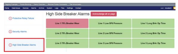
On this "High Side Breaker Alarms" page, one active unacknowledged alarm is shown.
