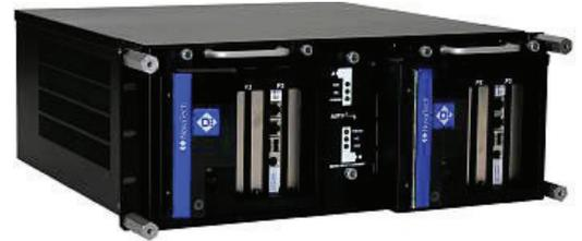
The PCM provides autonomous control over a portion of the process plant after the PCM's databases and programs are downloaded over the network. The PCM performs all continuous, sequential, and batch control functions and communicates with other D/3 nodes to support alarm, trending, and display functionality.
