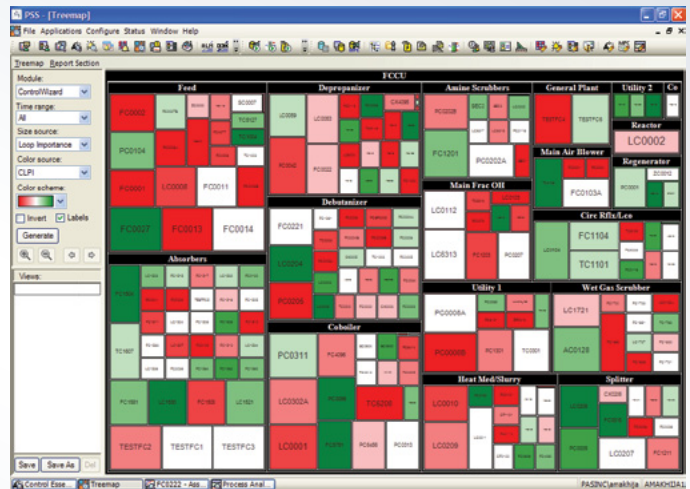
Control Loop performance is analyzed and arrayed by size and color for fast diagnosis and continuous improvement.
