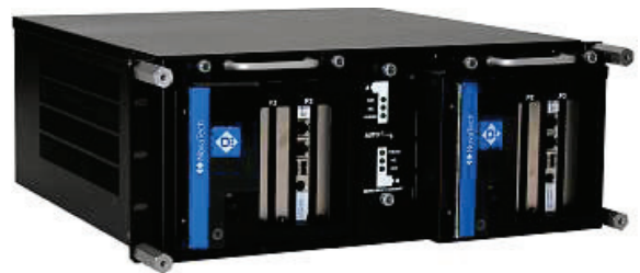
Rack mount chassis with two PCM 4100s
